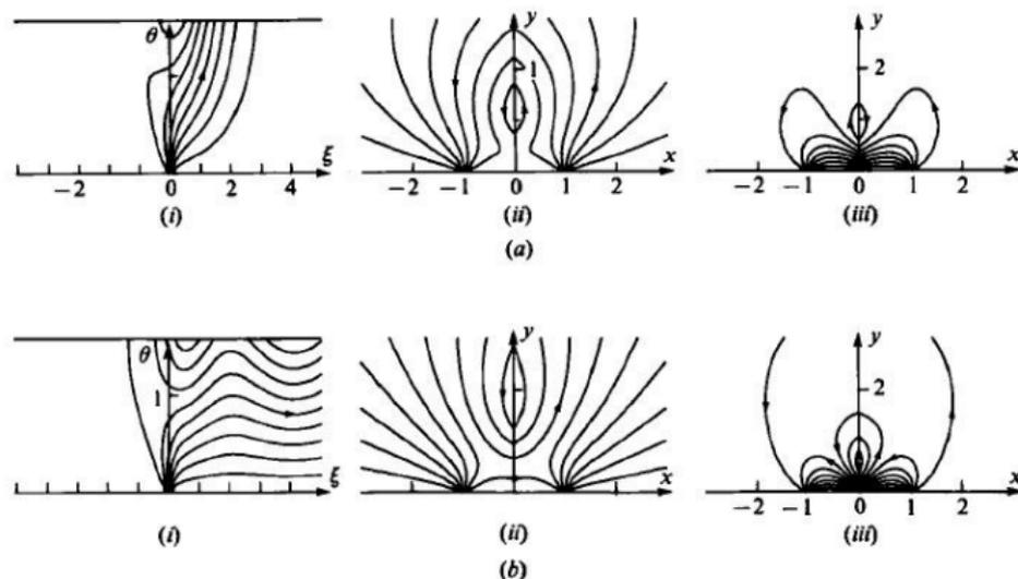
FIGURE 2. Streamline patterns at intermediate stages of the flow in figure 1. In both cases (i) gives the pattern in the  $(\xi, \theta)$ -strip, (ii) the pattern in the original coordinates for  $\gamma = 1$  and (iii) the pattern in the original coordinates for  $\gamma = -1$ . (a)  $t = 2$ ; (b)  $t = 10$ . The scales are as in figure 1.
