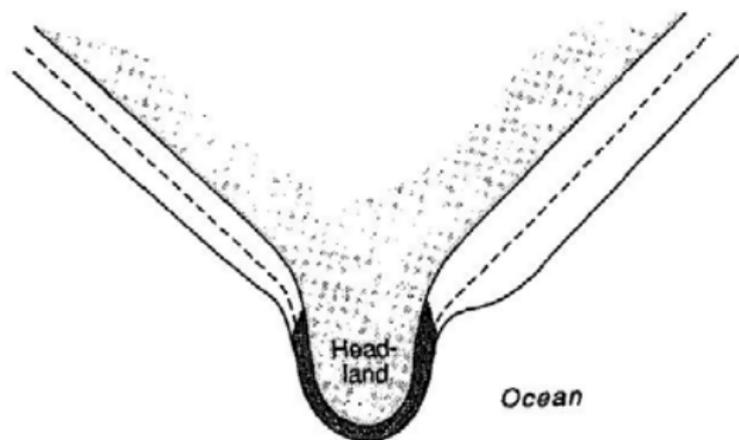
FIG. 13. Depth contours (in two dimensions) for a shelf interrupted by an arbitrarily large headland. When stratification is weak and frequencies are low ( $\omega \ll B \ll 1$ ), the EKW carries the entire incident mass flux past the headland. Any remaining incident energy flux is transported without loss by IKWs in high velocity layers of thickness  $N_0 H / f$  (shown shaded here) confined against vertical walls.
