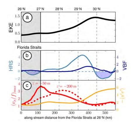
Model showing **barotropic instability** is the main source of eddy kinetic energy
