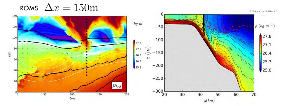
Density at bottom (colors), topography (black contours), bottom velocity (arrows) and free surface (white contours).
