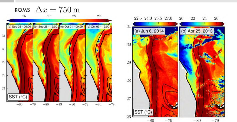
Observed SST showing cyclones on shoreward flank of Gulf Stream downstream from Florida Straits 1. Submesoscale instability and vortex street formation
