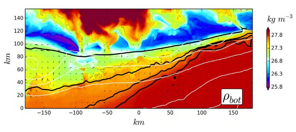
Density at bottom (colors), topography (black contours), bottom velocity (arrows) and free surface (white contours).
