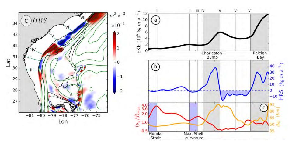
Conversion from mean kinetic to eddy kinetic energy (Barotropic instability)
