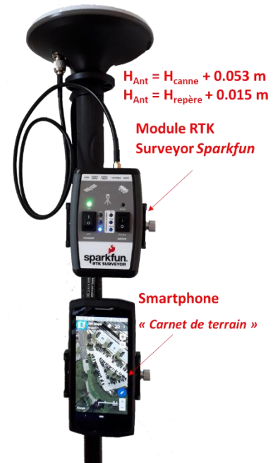
Figure 1 : Kit Rover (antenne mobile + module RTK Surveyor + Smartphone)
