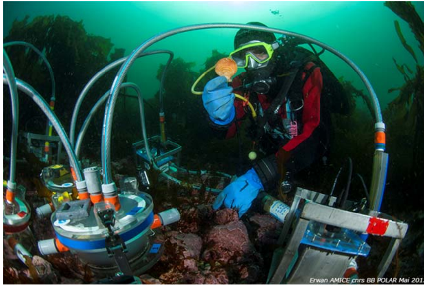
Figure 4: Benthic chambers used to measure respiration and filtration of Chlamys islandica during missions in Svalbard made in May and September 2013.
